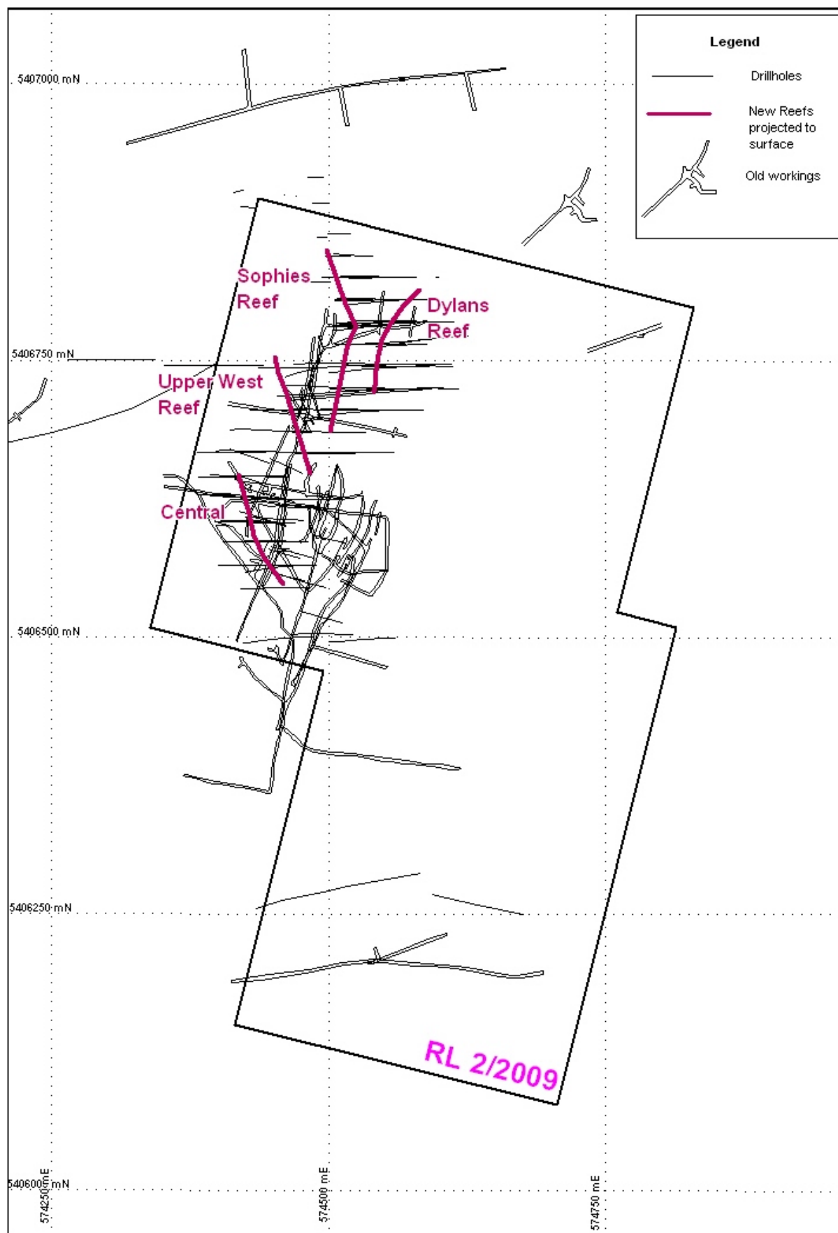
Figure 2: RL 2/2009 lease area with old underground workings, drilling and newly discovered reefs projected to surface
